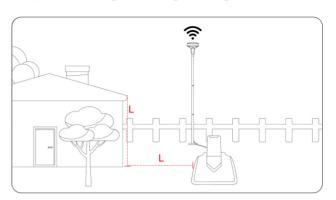
② Install the RTK installation components and connect the RTK base station to the charging station. Use an extension cable as needed.
